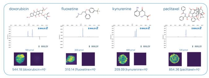
Figure 2: MALDI-2 increases sensitivity of steroids, doxorubicin, fluoxetin, kynurenine and paclitaxel. A single dilution of each of the four test compounds were spotted onto liver homogenate and imaged with MALDI-2 on and off. Use of MALDI-2 clearly provides higher sensitivity for the test compounds.
