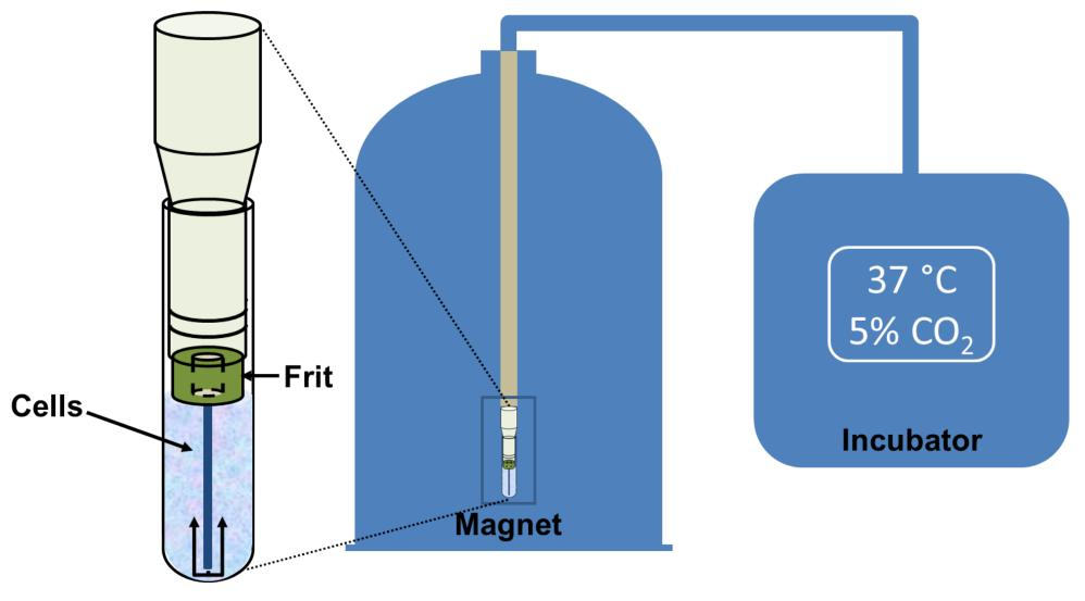
Flow unit with frit (modality B) to trap cells in the NMR tube. The system is equipped with a cell culture incubator for precise control of temperature,  $CO_2$  and  $O_2$  levels.
