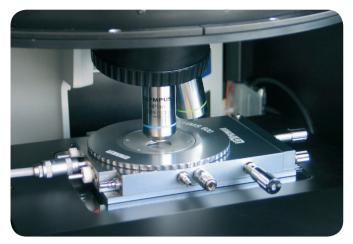
Abb. 4 Linkam stage in the sample compartment of the SENTERRA II<sup>(4)</sup>
