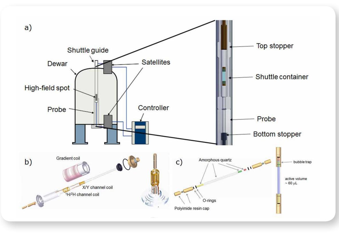
Fig. 2 Shuttle setup a) Pneumatic sample shuttling, b) Triple-resonance probe, c) Shuttle
